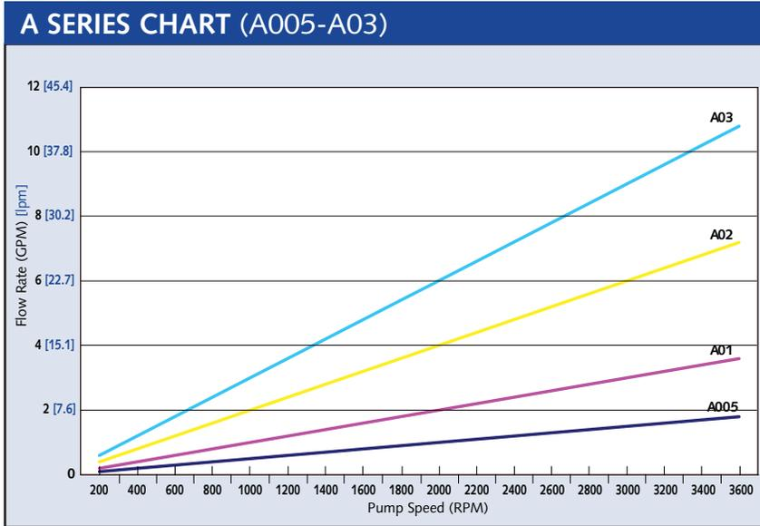
Performance figures show maximum horsepower requirements for minimum rated gallons per minute at the various speeds, viscosities and pressures. The charts are intended as a guide for conditions at the pump. In determining the proper conditions of operation for the pump, many factors must be considered including inlet conditions, liquid characteristics, and temperature.
