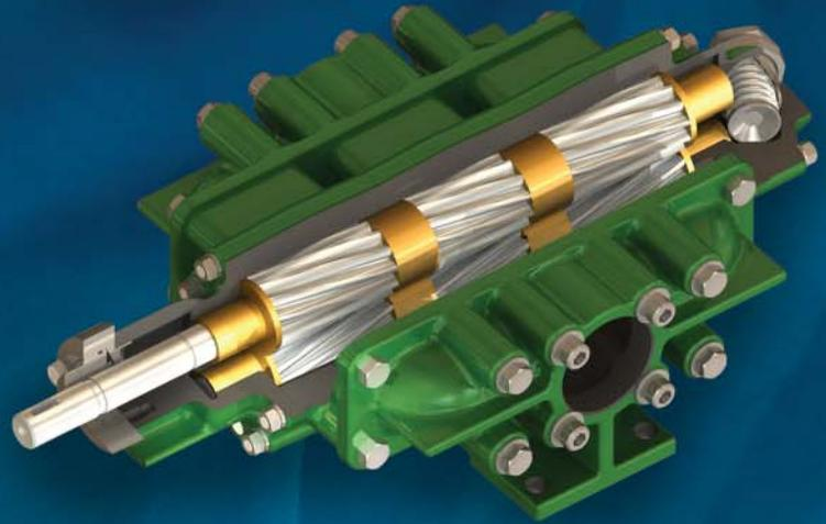
Roper AE Series pumps are well suited to applications where a compact and quiet unit is required, such as hydraulic lift applications. Bearings and wear-plates are special wear-resistant, high lead bronze. The pumping gears are accurately machined to run quietly and smoothly.
